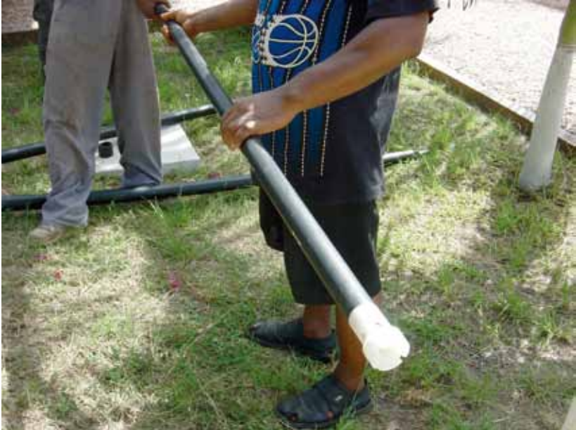
12. Connect the plunger rod (already assembled) to the pump rod.
