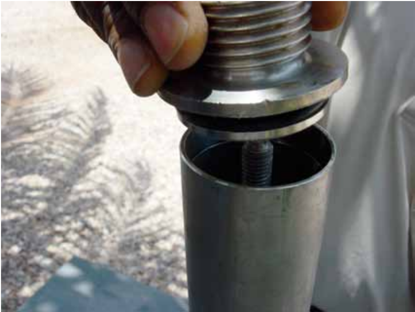
33. Connect the handle nipple to the handle T-bar.
