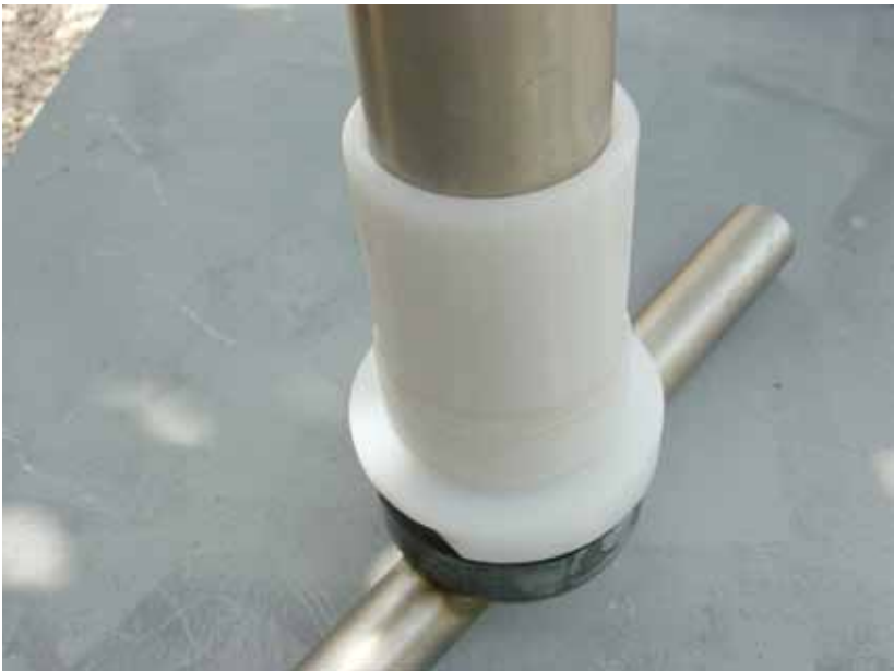
31.-32. Slide the sleevebearing on the handle pipe.
