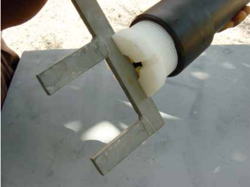
20. Fasten the bottom valve assembly to the coupled Riser pipe using the F-key.
