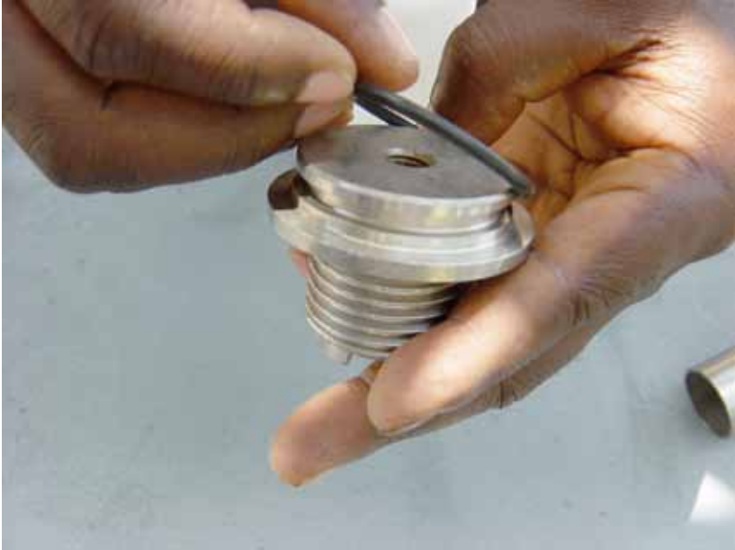
28. Place the o-ring in the grooved part of the handle nipple
