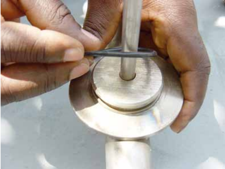
27. Place the o-ring in the grooved part of the handle T-bar.
