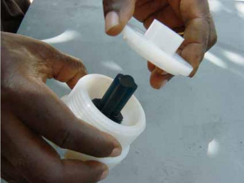
17.Ingiza plunger bottom valve (bobbin) kwenye bottom valve body.
