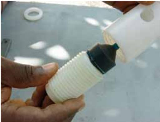
20. Ingiza bobbin kwenye plunger nipple na uifunge kwenye plunger body.
